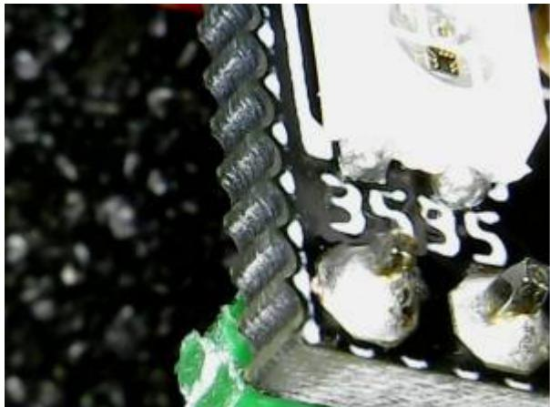
**Bild der fertigen Platine**
