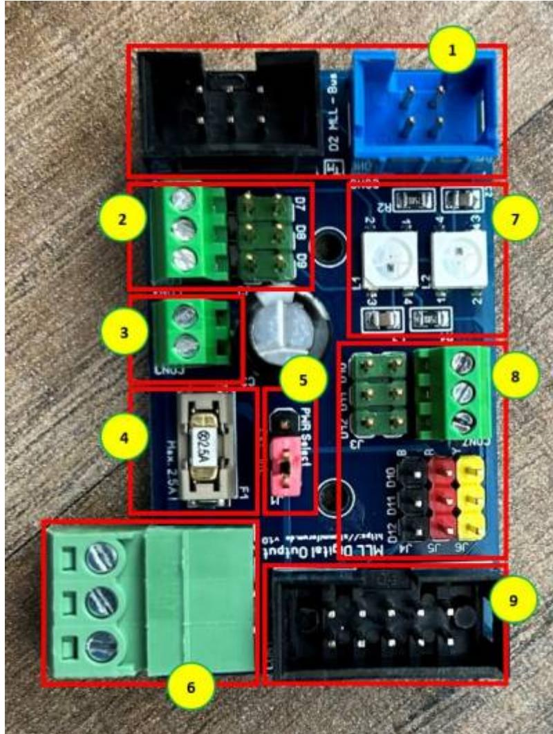
1. MLL Bus (D2) 6-pin (extra +12V) & 4-pin, both equal (parallel)
